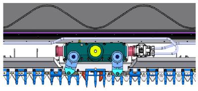
Center Knife Drive minimizes vibration of the cutter bar for smoother feeding.
